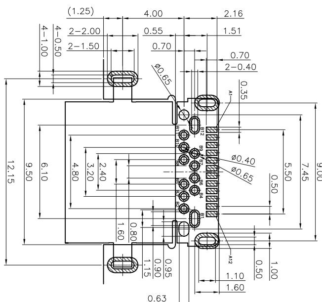
USB TYPE-C FULL-FEATURED RECEPTACLE INTERFACE PIN ASSIGNMENTS
